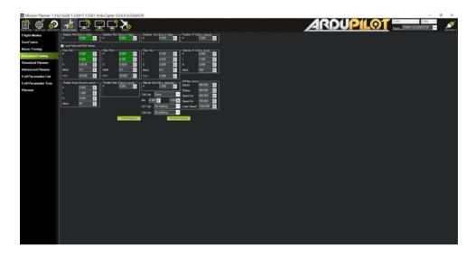
Here we changed the parameters as follows:-Stabilize Roll: P=6.5 Stabilize Pitch: P=6.5 Rate Roll: P=0.250, I=0.200 Rate Pitch: P=0.250, I=0.200
