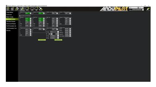
Here we changed the parameters as follows:-Stabilize Roll: P=4.5 Stabilize Pitch: P=4.5 Rate Roll: P=0.130, I=0.085 Rate Pitch: P=0.130, I=0.085
