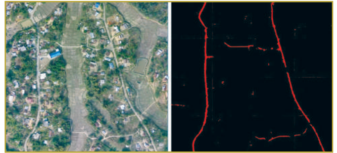
Extraction of roads using UNet from drone images
