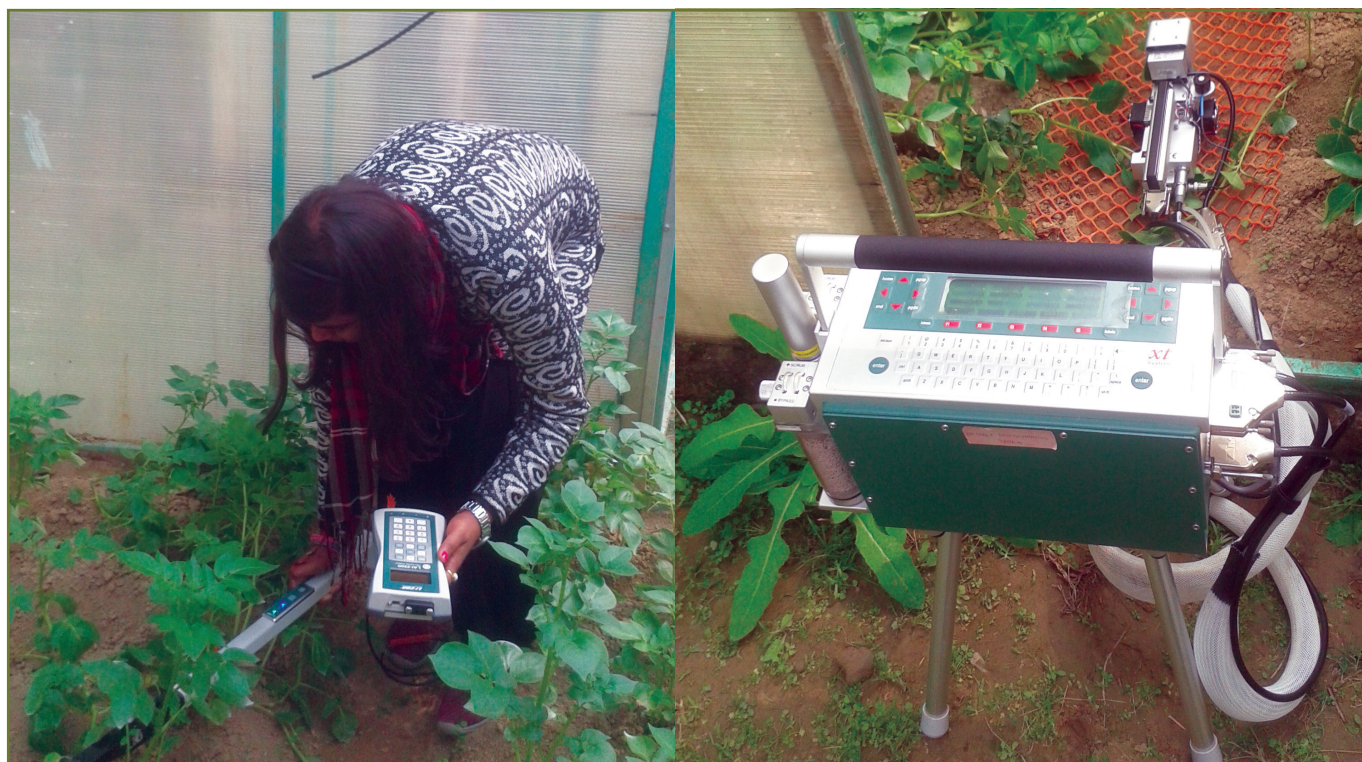
Figure 2.2: Biophysical parameter and spectral measurement of potato plantation using a LAI meter (left) and Photosynthesis measurement
