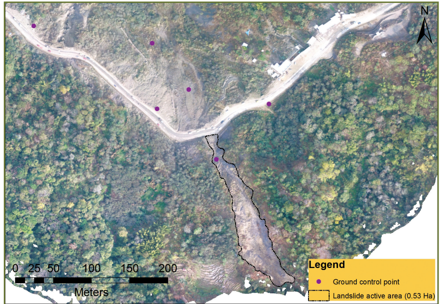
Figure 6.6: Ortho image of active landslide area along NH39 near Kohima, Nagaland
