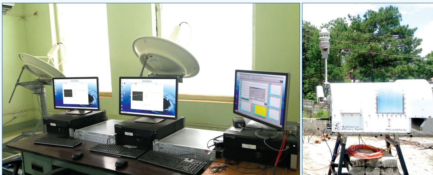
Two beacon receiver, parabolic antennas and receiver processor (20.2 GHz and 30.5 GHz), and 7-channel Ka-band humidity profiler radiometer installed at NESAC.
