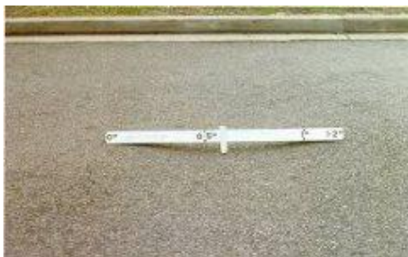
Figure 7: Depression. (Source: LGAM)
