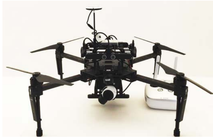
Figure 4: DJI Matrix 100 Quad-copter image.
