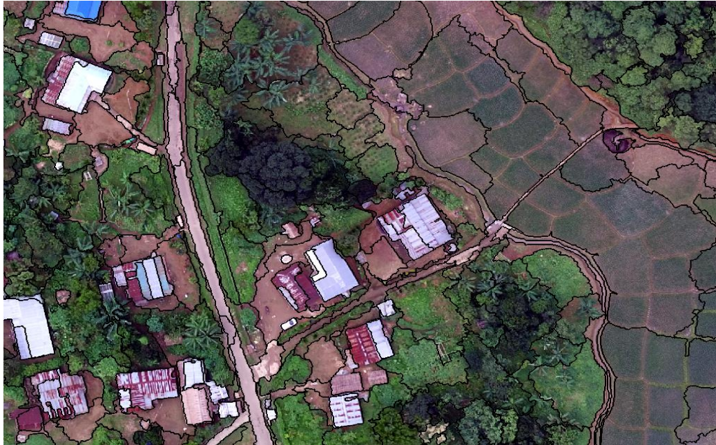
Figure 30: Final segmentation Result, M S: Scale-85 , Shape- 0.3 , Compactness-0.5 And SS :5
