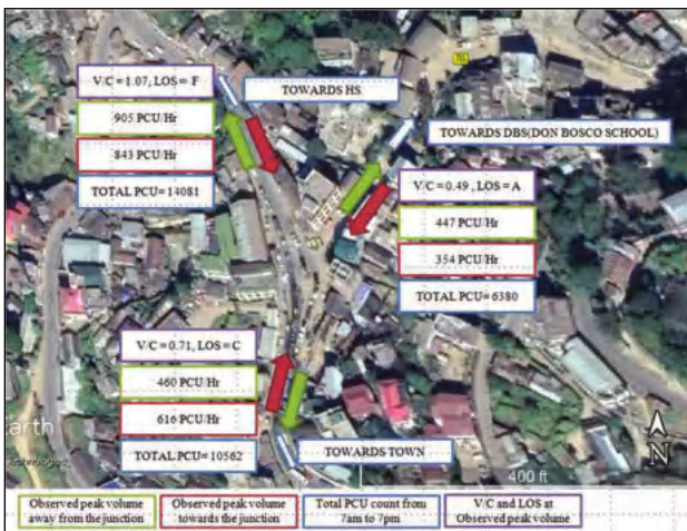
Volume/capacity ratio, LOS, observed peak volume away and towards the junction and total PCU count at Tinpatti junction
