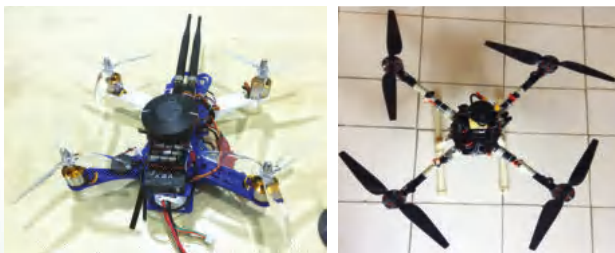
(a) 3D printed small Quadcopter (b) Assembled Quadcopter
