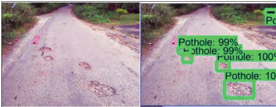
Automatic detection of potholes from the roads using DL embedded IOT device
