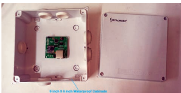
Water sensing node for measuring water level deployed at different location of Guwahati City
