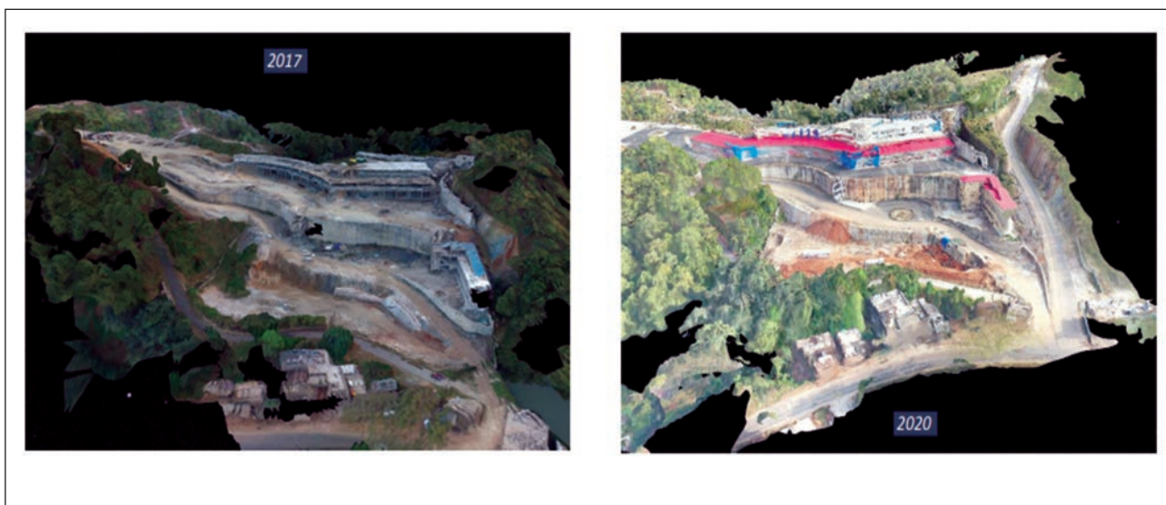
Tracking in 3D and assessment on the change quantification on high resolution multi-temporal UAV images
